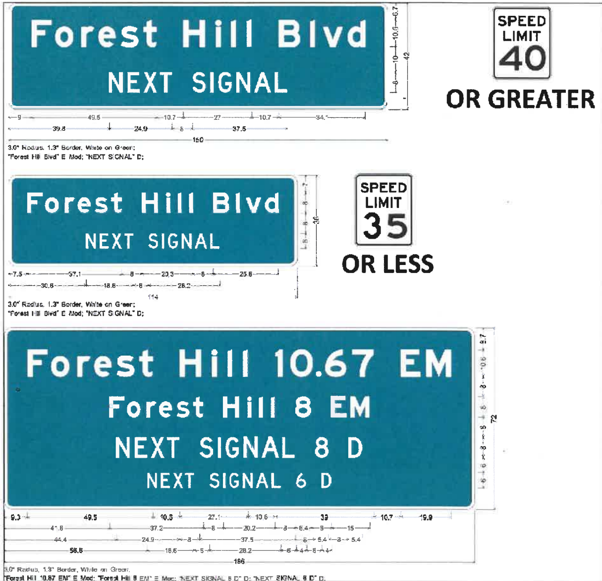
Figure 18 – 1 Examples of Advance Street Name Signs
